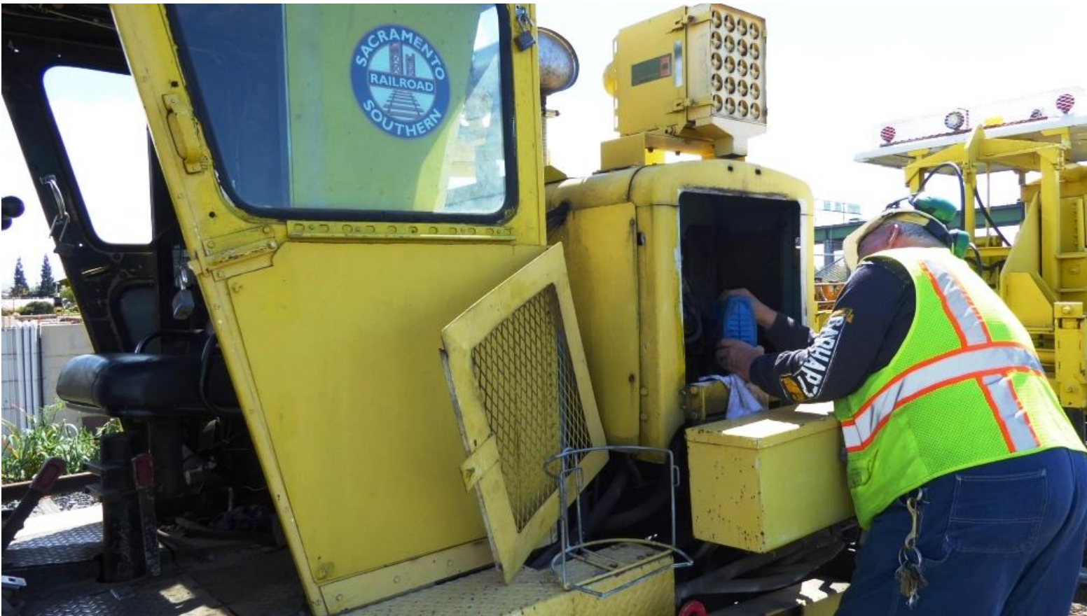
Harry adds oil to the scarifier-inserter
